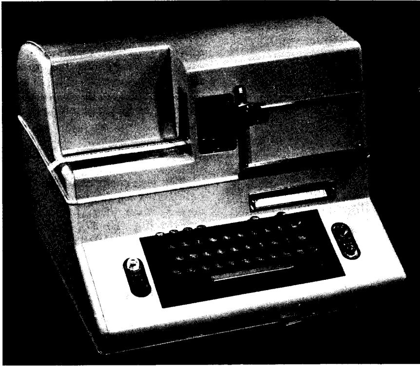
Figure 10-34.— Send/receive typing reperforator TT-253/UG. 50.116
